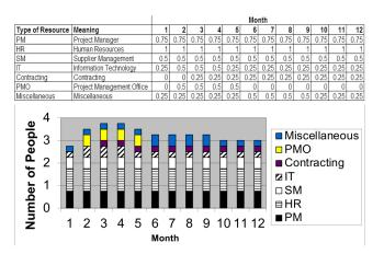
Figure 1.9: Sample Resource Histogram Broken Down by Type of Resource
