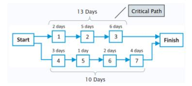
Figure 1.1: Network Diagram with Duration and Critical Path
