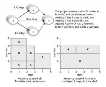
Figure 1.10: Resource Levelling with an AOA diagram, followed by graphs for usage if all activities start on day one versus delaying activity C by two days
