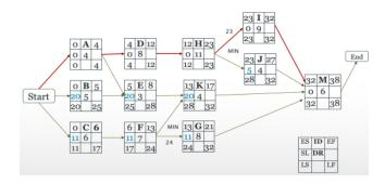
Figure 1.2: AON Diagram Produced from the above table
